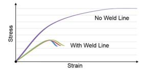
"The coupling of fill studies and FE analysis makes the predicted results more reliable. A detailed knowledge of the plastic material properties is important to design the products closer to the limits."
