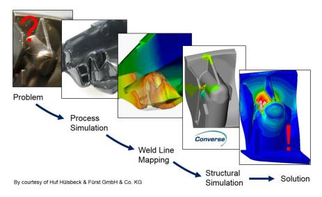
Especially but not only in fiber-reinforced plastic components detailed knowledge of material properties is essential. In addition to the fiber orientation and the mechanical properties the position of the weld lines must be very well known.
